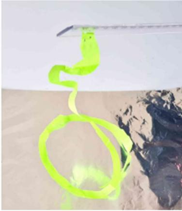
A tissue paper snake is placed on an aluminium foil. Then rub a plastic ruler with a synthetic fibre cloth and approach it to the snake's head. The snake straightens up & bites down.
